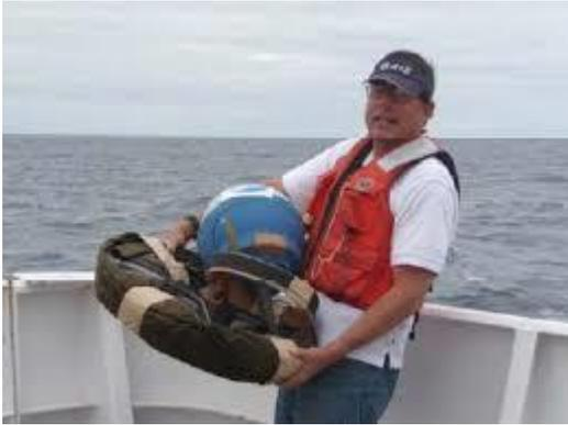
Drifters are buoys with instruments that float at the surface of the ocean and send their location data to satellites as they drift with the currents to provide scientists with information about how water moves. Scientists at the University of Miami spent two years testing various structures and materials before finalizing the new CARTHE drifter design, which is the first environmentally friendly drifter made from 85 percent seawater biodegradable components.
